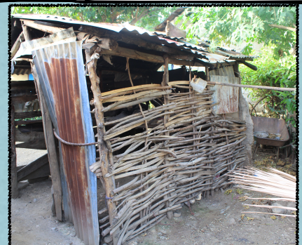
Pastor Oclane's outdoor kitchen. His home is constructed with the same type of sticks, then stuccoed.
